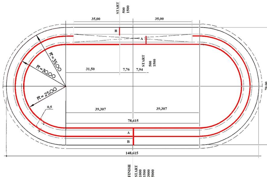
Reason: The inclusion of the 333m Standard speed skating track demarcation plan and respective information will facilitate the design of new rinks and the drawing of demarcation lines on existing ice rinks.
