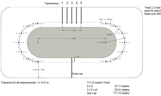
57.71 meters 53.41 meters 111.12 meters Track 2, 3 and 4 to be used for semi-finals and finals over 500 meters.
